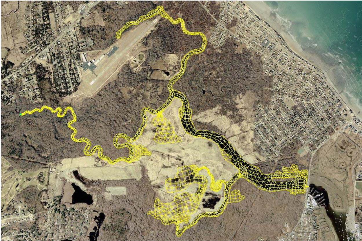
Figure 5. The yellow lines show the element boundaries of the numerical grid used for hydrodynamic modeling of Green Harbor.
