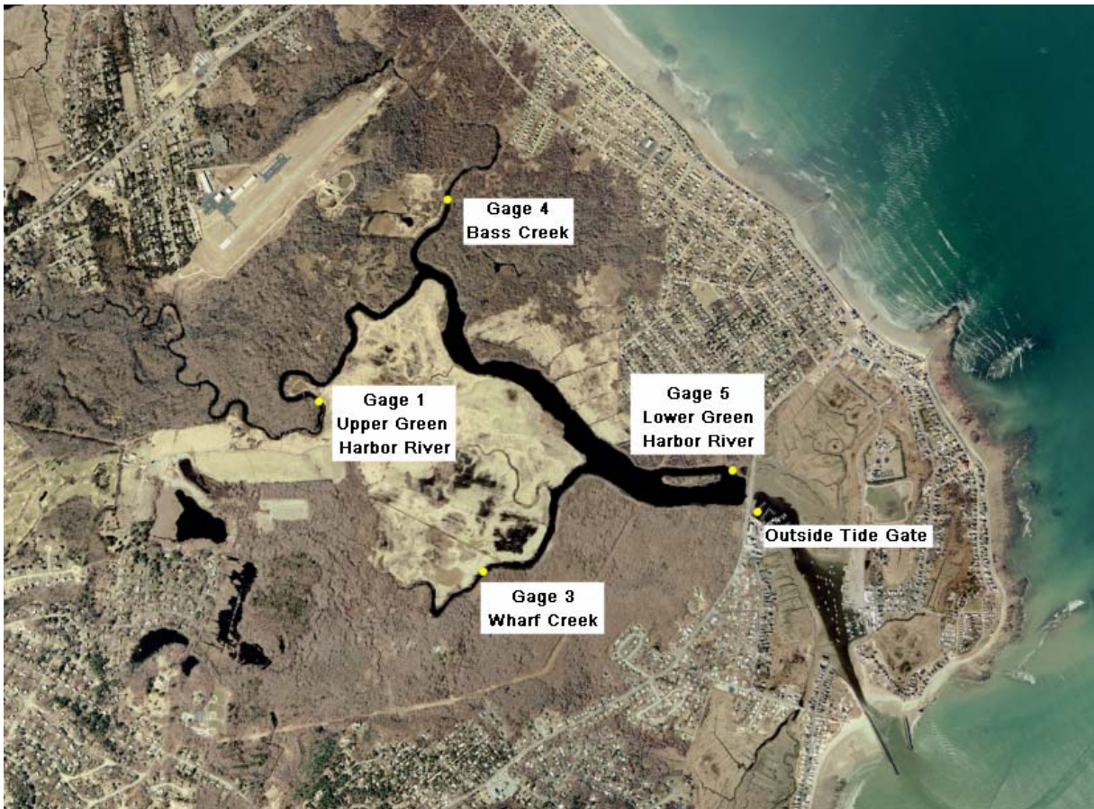
Figure 2. Map of the study region identifying locations of the tide gauges used to measure water level variations throughout the system. Gauges were deployed from late August to early October, 2006. Each yellow circle represents the approximate locations of the tide gauges.
