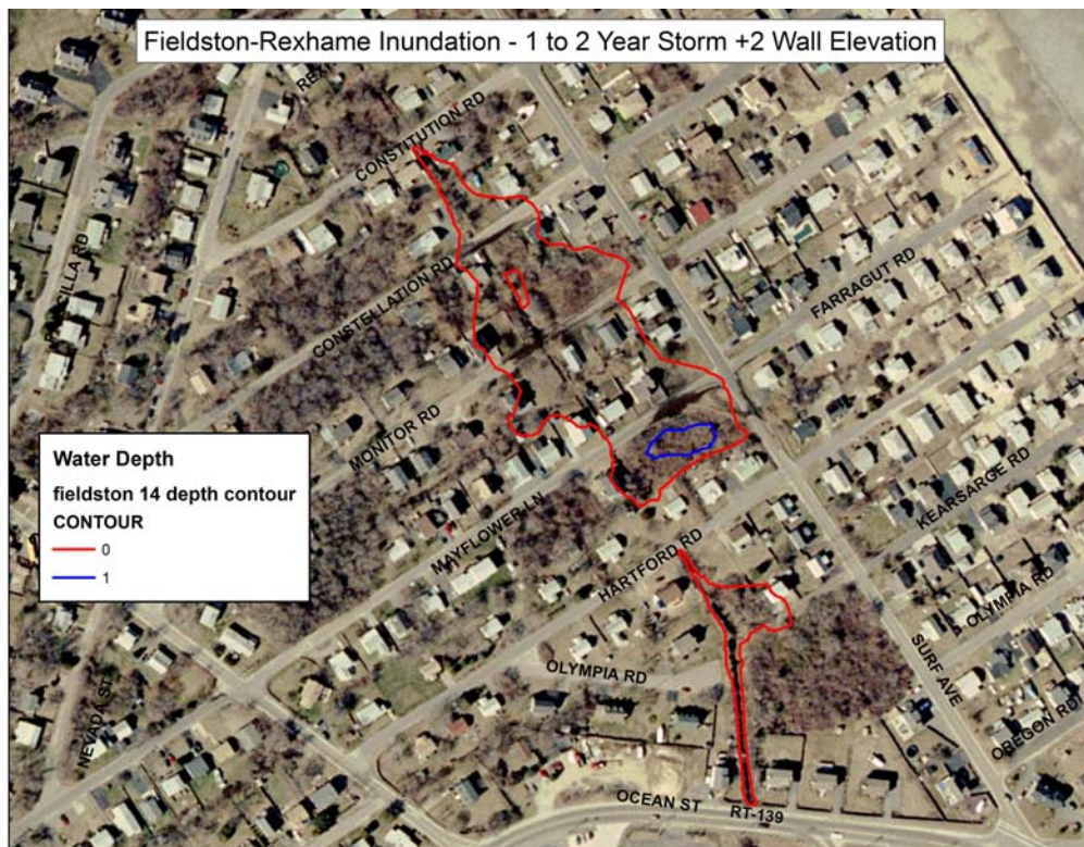
Figure 25. Fieldston Inundation for 1 and 2 Year Storm +2' on seawall
