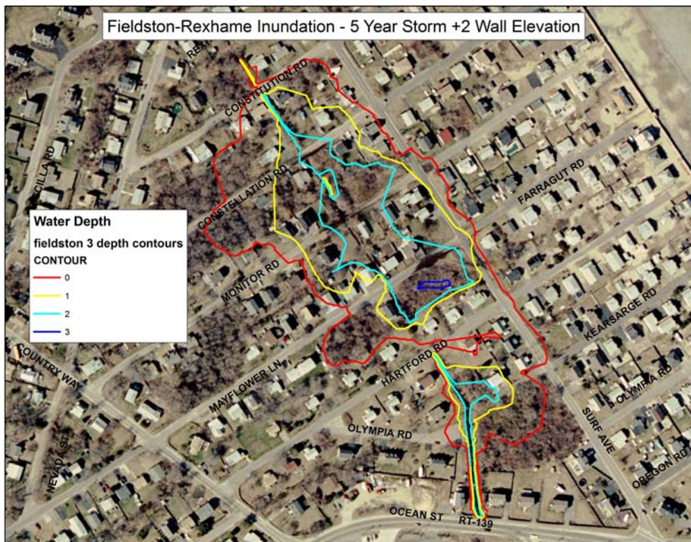
Figure 26. Fieldston Inundation for 5 Year Storm +2' on seawall
