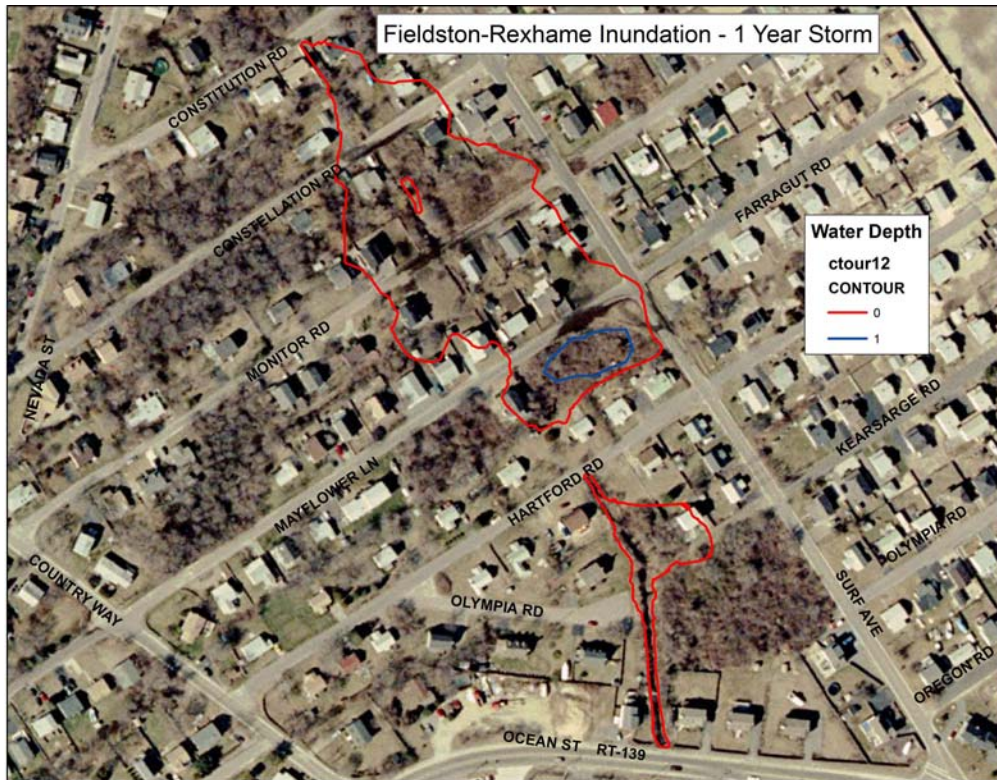
Figure 13. Fieldston Inundation for 1 year storm - existing conditions
